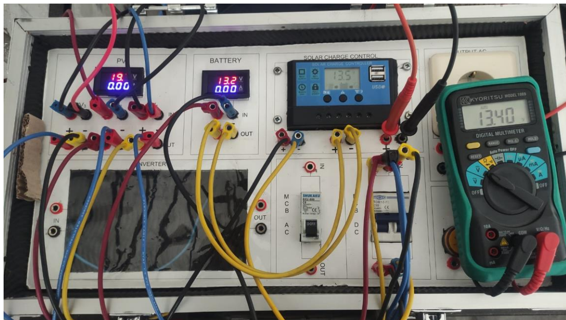
Gambar 12. Pengukuran Output Solar Charge Controller
