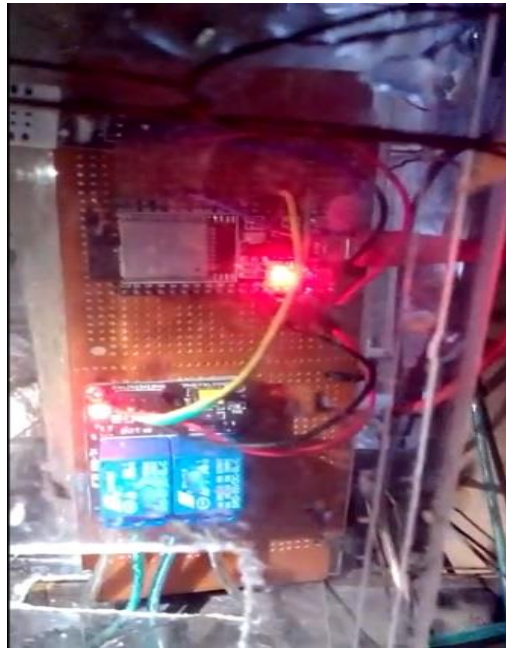
Gambar 8. Modul Relay 1 Menyala Pompa On Exhaust Off
