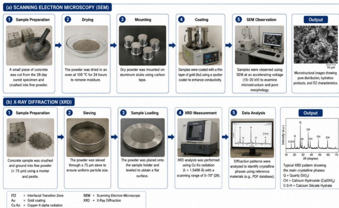
Figure 5. SEM and XRD Testing Procedures
