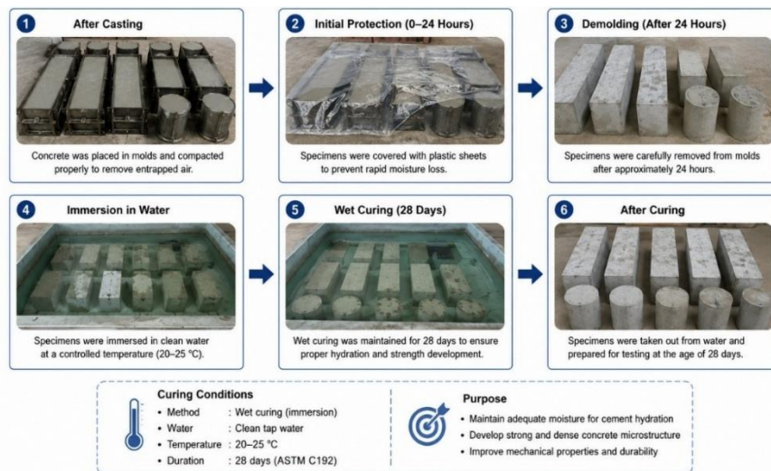
Figure 3. Wet Curing Process of Concrete Specimens
